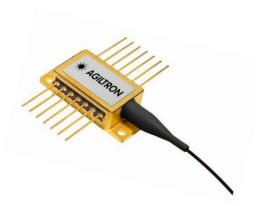
The 915nm series laser diodes are fabricated in a hermetically sealed 14-pin butterfly package. The laser diodes contain a monitor photodiode, thermoelectric cooler (TEC), and a thermistor to secure high-quality laser performance. Our laser products are Telcordia GR-468 qualified and in compliance with RoHS Directives.
